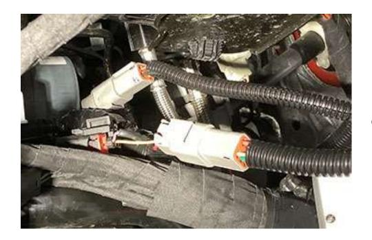
Connect the Tru-Speed to the two Deutsch connectors.
