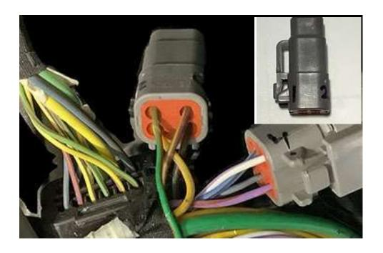
The four cut wires on the ABS connector are inserted into the Deutsch DTM06-4S in the order shown below. You will find it helpful to number the connector.
