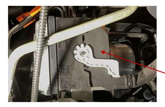
The ABS Module is located on top of the front axle spring tower, and accessible with the inner wheel liner removed.
