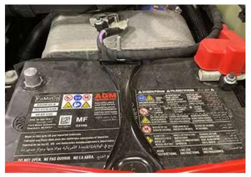
Disconnect the Negative Terminal at Batteries
