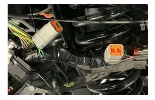
Using the electrical tape removed, retape the harness, leaving the two Deutsch connectors and the wheel sensor connector exposed.
