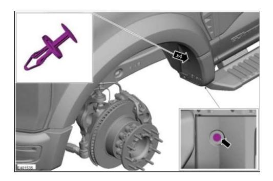
Remove the four push pins and the retainers attaching the wheel lip to the fender.
