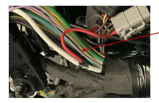
Locate the 10AWG white battery power wire and strip about 3/8" of insulation off the wire.
