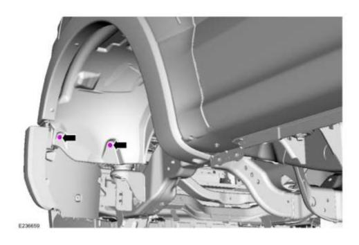
Using a 10mm socket, remove the bolt and push pin.
