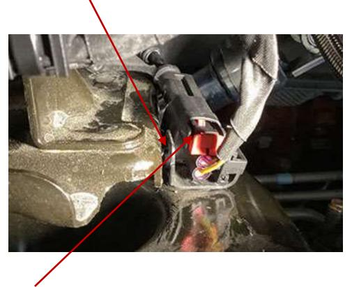
Separate the connector by sliding the red lock away from the connector and pressing the black tab behind it.
