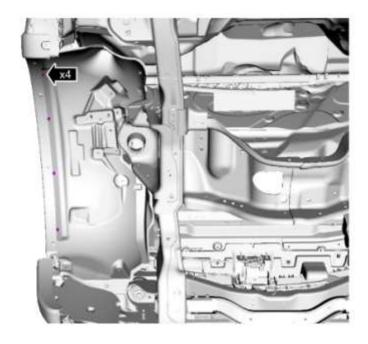
Using the 5.5mm socket, reinstall the four screws retaining the wheel liner to the fender.
