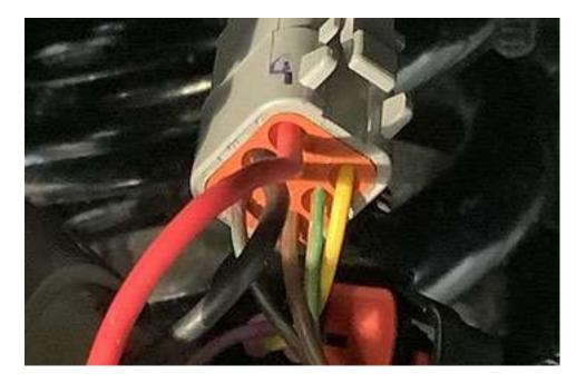
The four cut wires on the chassis side of the harness and the power and ground insert into the Deutsch DTM06-6S connector in the order shown below.
