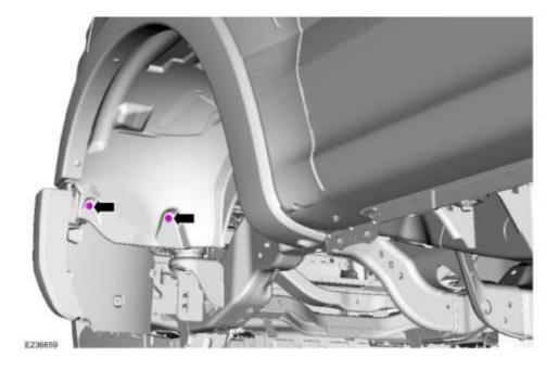
Using a 10mm socket, reinstall the bolt and pushpin.
