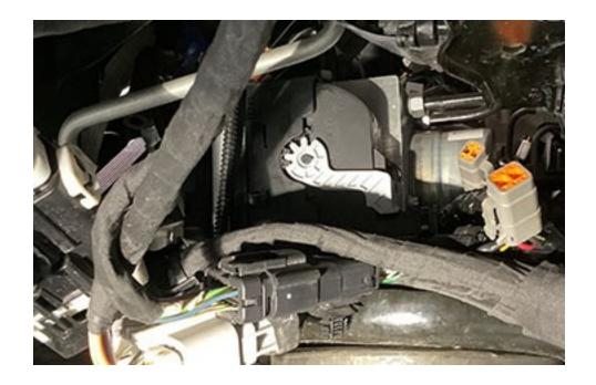
Reinstall the ABS connector as far as it will go pull the gray lever down. As the lever is pulled down the connector should pull into the ABS module. Pull the lever down until latches. Slide the red lock down.
