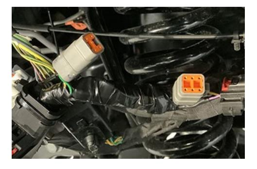
Using the electrical tape removed, retape the harness, leaving the two Deutsch connectors and the wheel sensor connector exposed.
