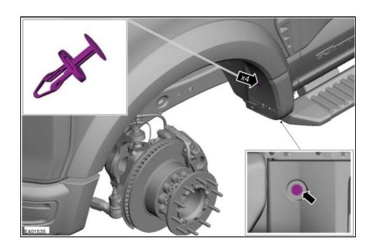
Reinstall the four pushpins and the retainers attaching wheel lip to the fender.
