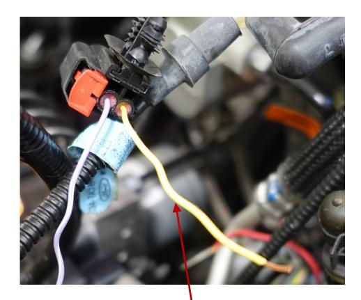
The pigtail attached to the two wire connector needs to be lengthen.
