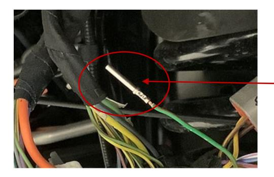
Install a Deutsch 0462-201-20141 pin on each end of the cut wires.
