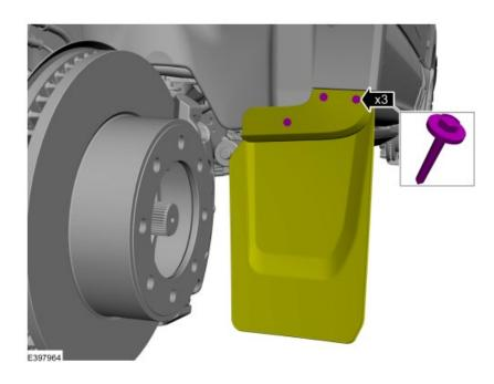
If equipped with mud flaps, use a 7mm wrench to remove the three bolts.
