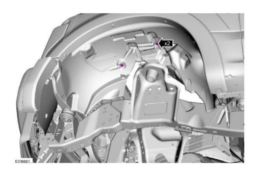
Using a 10mm socket, reinstall the two bolts.
