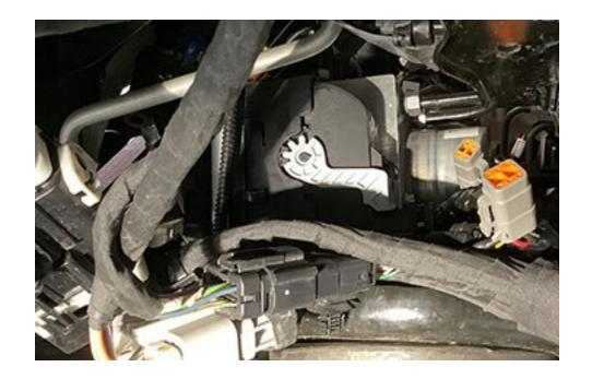
Reinstall the ABS connector as far as it will go, pull the gray lever down. As the lever is pulled down the connector should pull into the ABS module.
