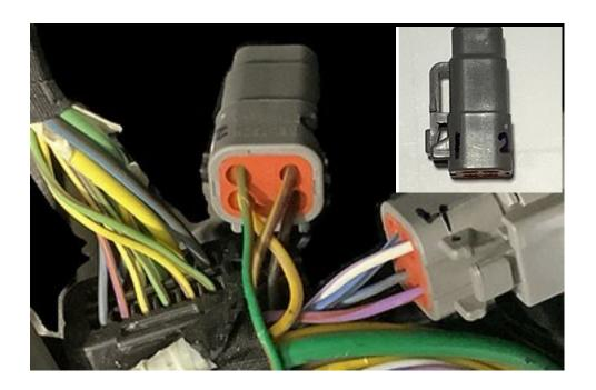
The four cut wires on the ABS connector side are inserted into the Deutsch DTM06-4S in the order shown below.
