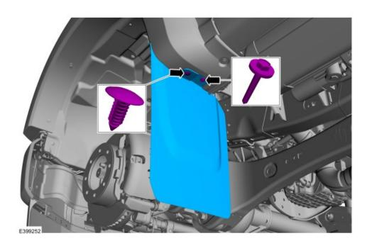
If equipped with mudflaps. reinstall the mud flap pushpin and bolt.
