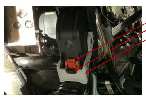
Remove the ABS connector from the ABS module.
