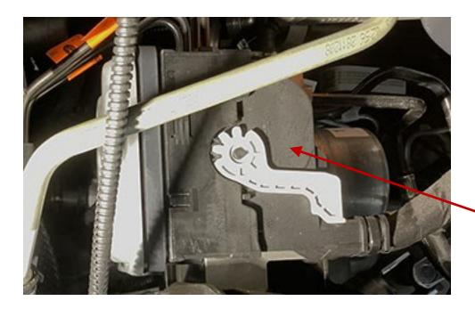
The ABS Module is located on top of the left front axle spring tower, and accessible with the left inner wheel liner removed.
