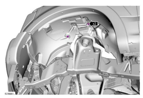
Using a 10mm socket, remove the two bolts.
