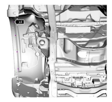
Using the 5.5mm socket, remove the four screws retaining the wheel liner.
