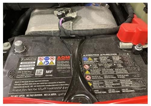
Disconnect the Negative Terminal at Batteries
