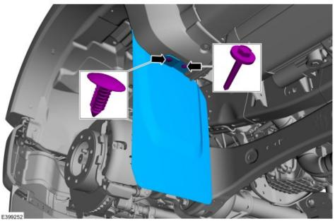
If equipped with mudflaps, remove the pushpin, bolt, and mud flap.
