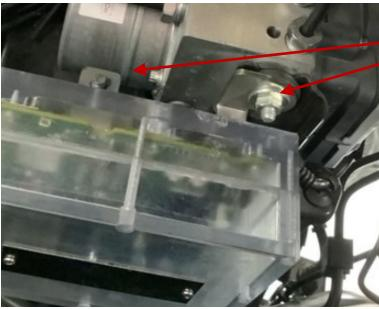
Install module on lower mounting bracket and ABS mounting stud.
