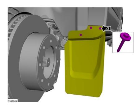
If equipped with mud flaps, use a 7mm wrench to reinstall the three bolts.
